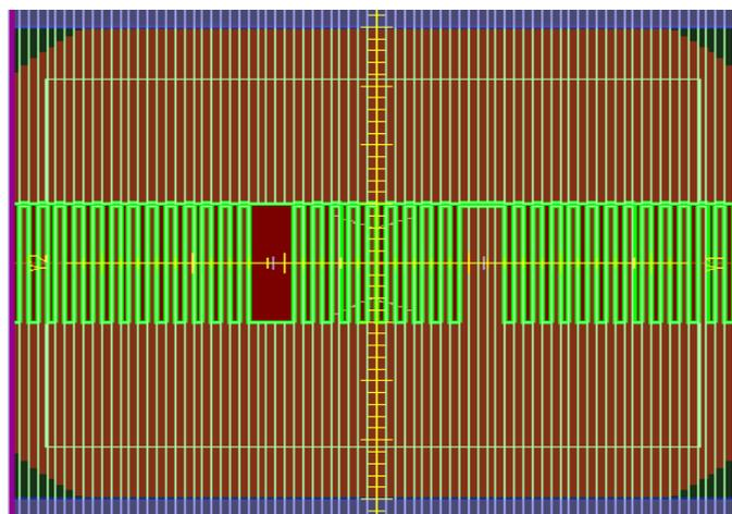
FIG. 2. BEV of the fields constructed to evaluate the LBROT value. The fields consist of a small field size (1-open leaf) to verify leaf bank rotation and one larger field size (5-open leaves) for dosimetric verification.
