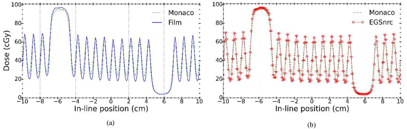
FIG. 12. Comparison of Monaco calculations against (a) EBT3 film measurements and (b) EGSnrc simulations for the field shown in Fig. 2.
