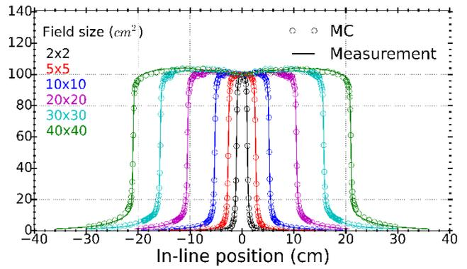
FIG. 6. Comparison of the measured and calculated (a) cross-line and (b) in-line profiles for various field sizes at 5 cm depth and 100 cm SSD.
